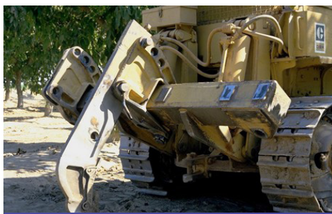
Figure 4. Deep ripping implements can be used to destroy old burrow systems (photo by Bob Beede, UCCE Emeritus.)
