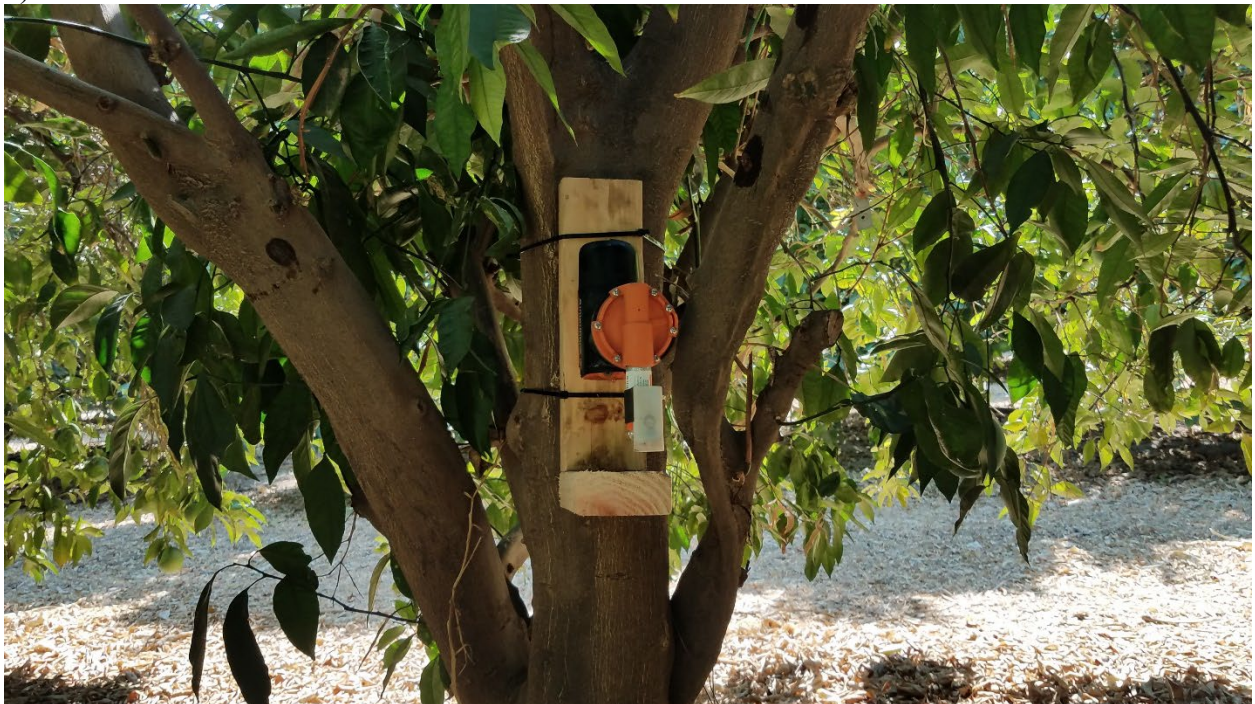
Figure 1. For three study sites, we attached Goodnature A24 traps to a wooden plank (a). The trap and plank were then attached to a tree via plastic cable ties. For one study site, we also included a wooden platform underneath the traps to allow better access to the trap for black rats (b).
