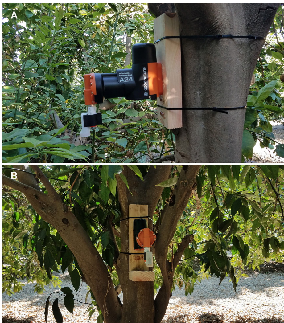
Figure 1. For three study sites, we attached Goodnature A24 traps to a wooden plank (A). The trap and plank were then attached to a tree via plastic cable ties. For one study site, we also included a wooden platform underneath the traps to allow better access to the trap for black rats (B).
