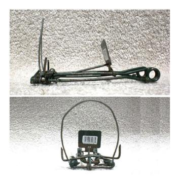
**Fig. 1.** Modified Macabee trap for capturing pocket gophers: side (top) and front (bottom) views. A strand of cable (1.6 mm in diameter, 23 cm in length) was attached to the front of the Macabee trap. The cable was formed into an upside-down U shape, with each end knotted (overhand knot) or twisted (strands separated then rejoined) onto either side of the trap anterior to the opposing pincer arms. The height of the attached cable was approximately 7 cm.
